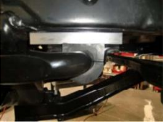
6. Sway bar spacer properly installed.
