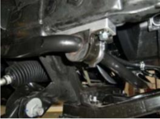
6. Sway bar spacer properly installed.
