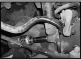
3. Working on the driver side, remove the stock sway bar from the frame mounting location. Save the hardware. Repeat procedure on the passenger side.
