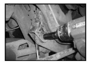
7. Working on the front driver side twin eye beam axle bracket, remove the stock bracket from the stock location. Save the stock hardware but the stock bracket may be discarded.
