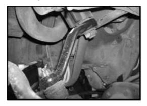
33. Slight adjustments may need to be done to the outer tie rods so the vehicle can be driven to an alignment shop. If this is the case on the vehicle that you are working on, loosen the stock hardware on the adjusting sleeve and using a pair of pliers, adjust the toe close enough so that the vehicle can be driven.
