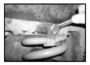
25. Locate the stock sway bar and the stock sway bar lower hardware. Working on the driver side, install the stock sway bar end link into the stock location and secure using the stock hardware. Do not tighten at this point. Repeat procedure on the passenger side. Let the stock sway bar hang.
