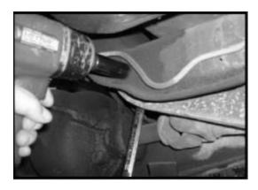
9. Working on the driver side stock radius arm bracket, remove the stock hardware or the stock rivets that connect the bracket to the frame rail. The stock hardware and rivets may be discard. Repeat procedure on the passenger side. Special note: Using a die grinder and making a cross cut on the rivets then using an air chisel will help make the removal of the rivets easier.
