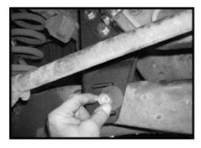
15. Locate the new rear twin eye beam axle pivot relocation bracket and the stock hardware. Install the new rear twin eye beam axle pivot relocation bracket into the stock location and secure using the stock hardware. Make sure to use thread locker or loctite and torque to 75 ft lbs. Special note: Make sure that the new twin eye beam axle pivot relocation bracket is seating square into the stock location.
