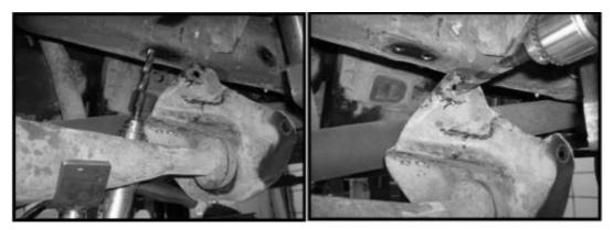
21. Locate the driver and passenger side radius arm relocation brackets. Locate (8) 1/2" x 1 1/2" bolts, (16) 7/16" USS flat washers and (8) 1/2" unitorque nuts from hardware bag. Working on the driver side, install the new radius arm relocation bracket into the stock location and secure using the new 1/2" x 1 1/2" bolts and hardware. Do not tighten at this point. Repeat procedure on the passenger side.
