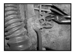
36. Working on the driver side, carefully pull the hard line out so that the new front brake line relocation bracket can be installed. Repeat procedure on the passenger side. Special note: Take special care not to damage the stock brake line when performing this step.
