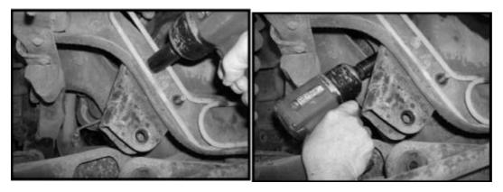
8. Working on the rear passenger side twin eye beam axle, remove the stock mounting hardware that connects the rear axle to the stock location. Save the stock hardware.
