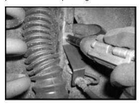
39. Locate (2) e-clips from hardware bag. Working on the driver side, install the new e-clips to the stock brake line on the back side of the newly installed brake line relocation bracket. Repeat procedure on the passenger side. Special note: Once the completion of the suspension system has performed and the weight of the vehicle is on the ground, check to make sure that the stock brake line does not rub on the inside of the tire.
