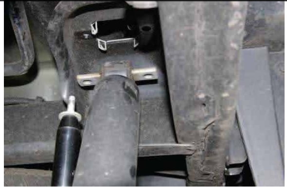
Disconnect upper shock mounting bolts
