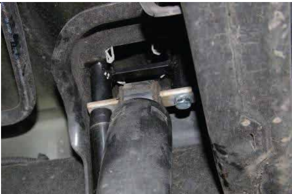
Install upper shock extensions and new hardware.
