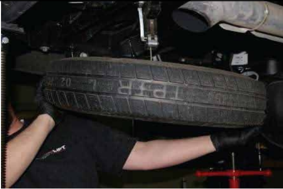
Remove spare tire in order to remove shackle bolts
