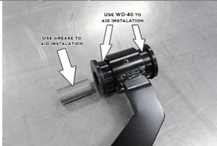
Figure 2: Bushing and Crush Sleeve installation
