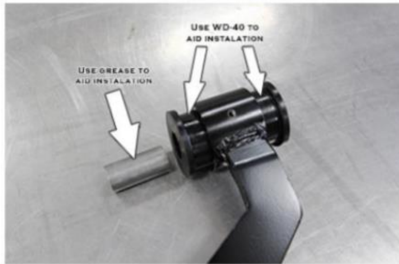
Figure 2: bushing and crush sleeve installation
