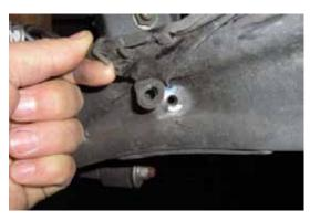
16. Unbolt the lower sway bar end link with a 14mm socket.
