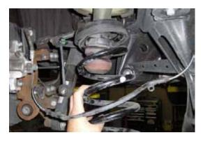
23. Use a 14mm socket and extension to remove the rear bump stop bracket.
