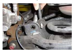
17. Support the lower control arm with a jack. Remove the rear upper shock mounting bolt.
