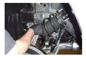
8. Please note that the strut extensions are driver side and passenger side specific. Arrow points toward front of vehicle
