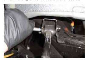
20. Adjust the EZ Arm to the same length as the stock arm. Install the arm by first installing the bolt at the body, but DO NOT TIGHTEN. Install the ball joint end into the knuckle using the OEM nut and cotter pin.
