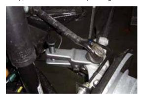
19. Remove the bolt on the body end of the arm and remove the stock arm. Make sure that both ends of the EZ Arm have equal thread showing on both sides of the turnbuckle.
