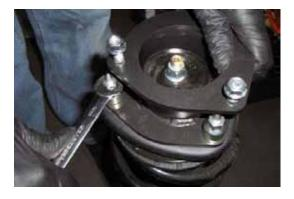
10. Install strut back into factory location, install nuts supplied with kit but leave loose.
