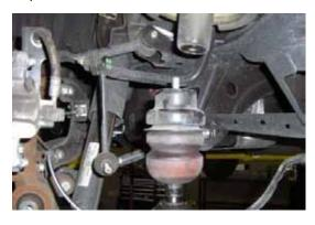
24. The rear coil spacer will mount in the factory coil bucket.
