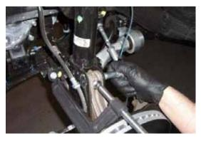
12. Tighten the three upper strut mounting nuts (14mm) 30 lb-ft.
