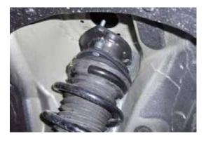
11. Insert the knuckle into the lower strut mount. A C-Clamp may be needed to align the mounting holes. Insert the OEM hardware and tighten to 200 lb-ft.
