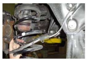
27. Use a jack to raise the lower control arm, align the mounting holes and install the OEM bolt. Tighten to 117 lb-ft.
