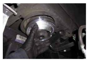
25. Reinstall the bump stop and bracket with the coil spacer on top.
