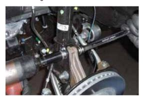
7. Carefully remove the strut from the vehicle making sure not to drop it on the outer CV boot. Tilting the knuckle towards the rear of the vehicle will make removal easier.
