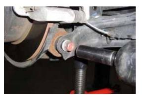
22. Lower the jack then remove the coil. Be sure to mark where the spring seat is on the lower control arm. You may need to loosen the cam bolt at the frame.
