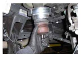
26. Push down on the lower control arm and install the coil. Make sure that the coil is properly seated in the lower control arm.
