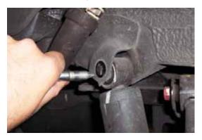
18. Remove the nut and cotter pin from the outer ball joint end of the upper arm and break the taper using a tie rod end separator.
