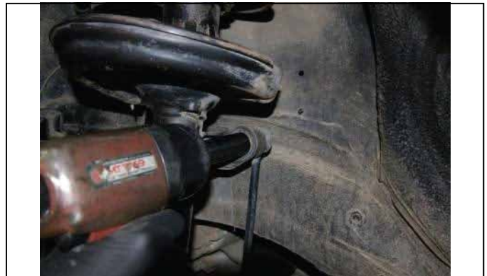
Disconnect and remove front sway bar end links
