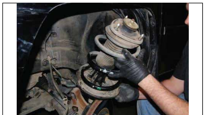
Lower suspension and remove strut. Caution: CV boot
