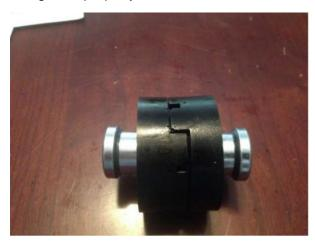
3. Install threaded ring and tighten using supplied spanner wrench. It may be helpful to apply a small amount of grease onto threads before installation. Once tightened, ensure that one of the grooves in the threaded ring is aligned with the set-screw hole.
