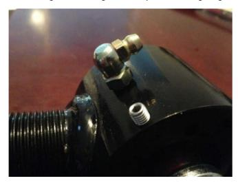
6. Thread jam nut onto flex joint housing and thread flex joint into control arm. Do not tighten jam nut at this point.
