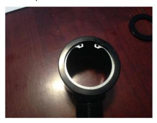
2. Insert one bushing half into flex joint housing. The flat side of the bushing should rest against the flat washer. Apply a small amount of grease to inside of each bushing half and onto center ball. Insert bushing center ball into bushing half. Insert second bushing half into housing. It is important that the two busing halves fit together properly, as demonstrated in the next photo.
