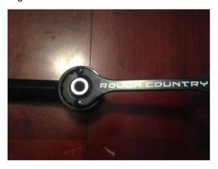
4. Insert set-screw into outer hole on housing end as shown in next photo. Tighten with 3/32" allen wrench. This locks the threaded ring into place, ensuring that it does not come loose over time.
