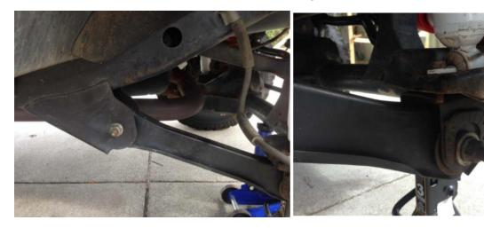
9. Using a tape measure, measure the length of the stock control arm. This measurement should be taken from the center of each eyelet in the control arm as shown in the picture below.
