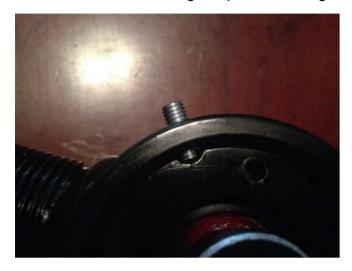
5. Install grease fitting into flex joint housing. Tighten using 3/8" wrench.
