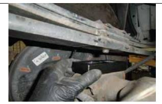
Place new block into position (1.0" block shown)
