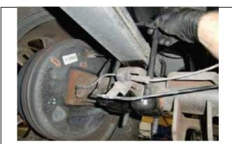
Remove u-bolts and axle mounting plate
