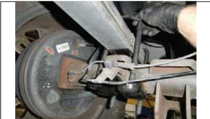
Remove u-bolts and axle mounting plate
