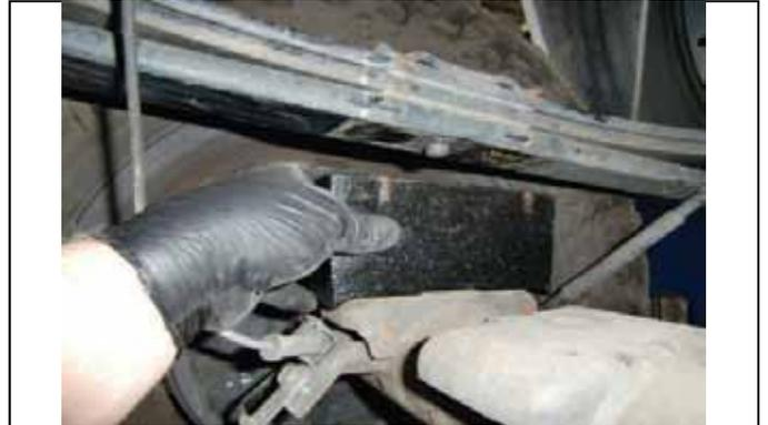
Shown (3.0" block) replacing factory block on 4WD models
