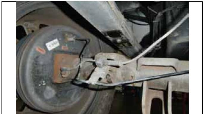
Carefully lower axle enough to install new block
