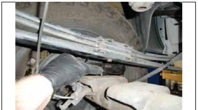
4WD models lower axle and remove factory block
