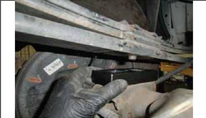
Place new block into position (1.0" block shown)
