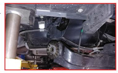
Once the control arm is lowered enough, remove the rear spring from the frame. Note the orientation of the lower spring pig tail and the locking tab on the lower isolator for reinstallation.
