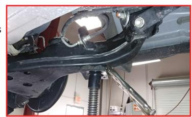
Remove the lower control arm cam bolt. Lower the control arm down while watching the brake line for binding or stretching. Adjust as necessary.
