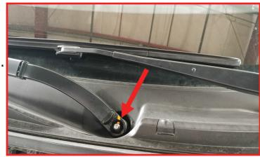
Locate the 6 plastic clips holding the cowl to the body. Remove all the clips and set aside. Gently lift up on cowling from the engine bay side, while lifting pull towards the front of the vehicle to disengage from the windshield. Once disengaged from the windshield, set aside in the engine bay.
