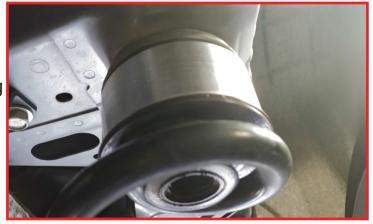
Use the jack on the lower control arm to raise the pivot back into the frame pocket. Use of a helper to pull on the suspension to line up the holes will aid in installation. Install the cam bolt from the back to the front (opposite of the way it was removed). This is not necessary, but can make installation easier.
