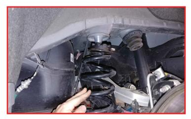
Install the rear spring spacer on top of the factory isolator. Install the spring back into the vehicle. Make sure the lower spring is orientated to the spring lock on the lower isolator.
