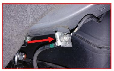
Gently pull on the brake line ferrule and slide the metal brake line through the mount. This is done to give slack for lowering the control arm. Do not bend or mangle the metal line.
