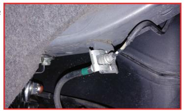
Once both sides of the vehicle are completed, raise the sway bar up and install to the frame using the factory hardware and clamp. Torque to 30 ft-lbs.
