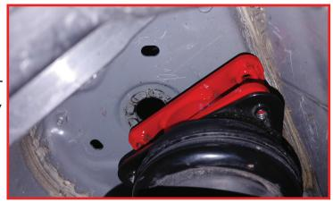
Use of a stubby wrench with a ratcheting head is recommended. Torque to 15 ft-lbs. You may have to use a crows foot wrench head and extension to gain access for the torque wrench. Raise the suspension using the jack while lining the upper strut extension up with the bolt holes on the strut tower. Use of a helper will aid in the installation. Install the strut assembly to the strut tower using the provided 3/8" bolts. Once all three bolts have been started, torque to 30 ft-lbs.
