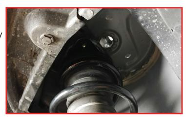
Install the strut extension onto the factory top hat using the factory hardware. This is a tight fit to get the bolts into place. The top hat can be rotated to access the bolts. Once all have been started, tighten all down.
