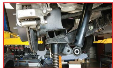
Loosen but do not remove the control arm hardware at the knuckle and the sway bar end link at the sway bar and lower control arm. This is to allow the full droop without binding the rubber bushings.
