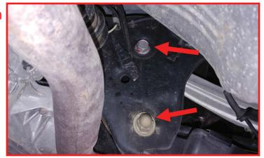
Move the jack to the front of the lower control arm. Use of a pair of locking pliers in the front drain hole will aid in keeping the jack from sliding up the arm.
