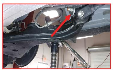
Once the lower control arm is installed into the frame pocket, move the jack to the back of the control arm and raise the arm enough to install the rear shock hardware. Do not tighten at this time.
