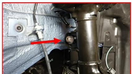
Remove the brake line bracket at the strut body. Let hang out of the way.
