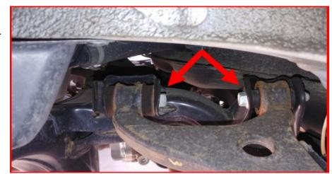
Loosen but do not remove the front lower control arm bolt at the subframe.
