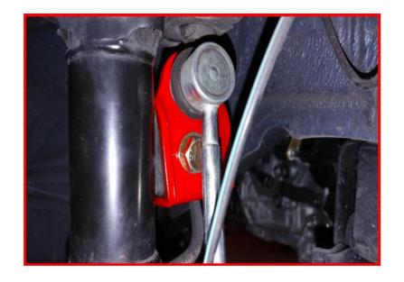
Install the front wheels and lower the vehicle to the ground. Torque the lug nuts to the wheel manufacturers specs. Jounce the front end to settle the suspension. Torque the upper strut spacer to 30 ft-lbs.
