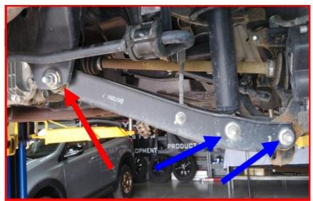
Lower the control arm down and remove the strut from the vehicle and let the control arm hang.
