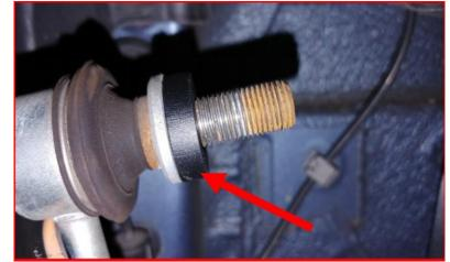
Install the factory end link to the bracket using the factory hardware. Torque the bracket and end link to 45 ftlbs.
