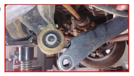
Install the sway bar brackets to the subframe using the provided M8 counter sunk bolts and a drop of thread locker. Torque to 25 ft-lbs.
