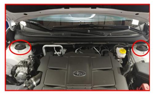
Locate the front strut extension. Install to the top of the strut using the factory hardware. Torque to 30 ft-lbs. Drill out the 6 strut mounting holes in the strut tower with a 27/64" drill bit. Paint exposed metal with a high quality rust preventative paint.
