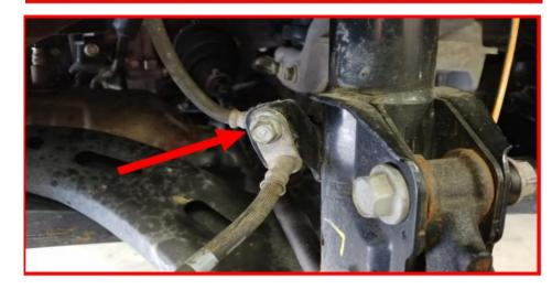
Install the sway bar bracket to the strut using the provided M12 bolts, washers, and nuts. Do not tighten at this time. If you have not started the opposite side of the vehicle at this time, you may not be able to line the sway bar up until the opposite side is released.
