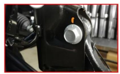
Install the brake line bracket to the strut body using the factory hardware. Torque to 5 ft-lbs. Install the ABS wire clip back to the strut.
