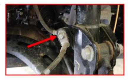
Install the sway bar bracket to the strut using the provided M12 bolts, washers, and nuts. Do not tighten at this time. If you have not started the opposite side of the vehicle at this time, you may not be able to line the sway bar up until the opposite side is released.
