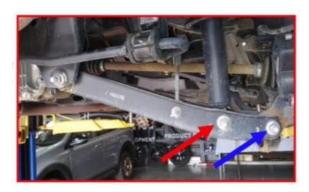
Install the lower front control arm to the knuckle using the factory hardware. Do not tighten at this time.
