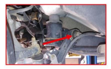
Remove the front lower control arm bolt at the knuckle. Let the control arm hang out of the way. This is for access to the rear lower control arm bolt removal.
