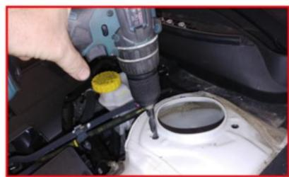
Install the completed strut assembly to the strut tower using the provided M10 flange nuts. Leave loose to aid in installation of the knuckle. A helper is recommended. Passenger side shown. The spacers are offset to the inside and rear of the vehicle to adjust for camber and caster. THEY MUST BE INSTALLED AS SHOWN.
