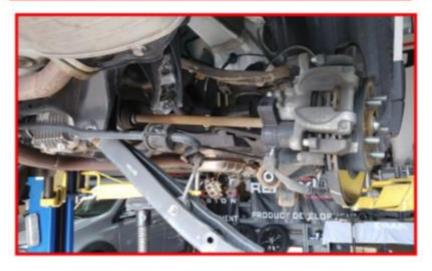
Locate the strut extension. Install using the factory hardware. You will have to start each nut before tightening fully. Run each nut down in an alternating pattern until you can torque them down. Torque to 30 ft-lbs.
