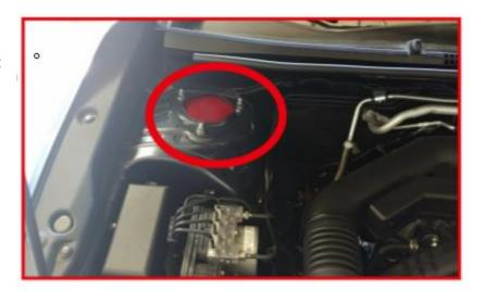
Jack the rear of the vehicle up and place jack stands under the main lifting points indicated by the owners manual. Open the hatch and remove the spare tire cover / carpet. Remove the two outer carpeted covers closest to the fender wells and set aside. Remove the 4 strut mounting nuts.
