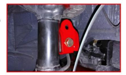
Install the 1/4" thick spacer washer onto the end link.
