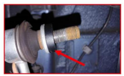
Install the factory end link to the bracket using the factory hardware. Torque the bracket and end link to 45 ftlbs.
