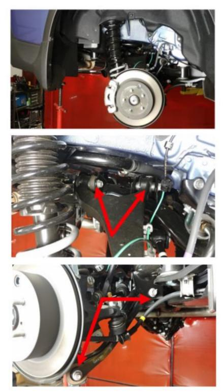
Loosen but do not remove the upper control arm bolts.
