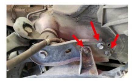
Loosen driver side cradle-to-body bolts. Remove passenger side cradle bolts. Lower the cradle until the billet spacers fit between body and OEM spacers on passenger side. Reinstall passenger side bolts, but do not tighten at this time. Remove driver side bolts, and repeat process.
