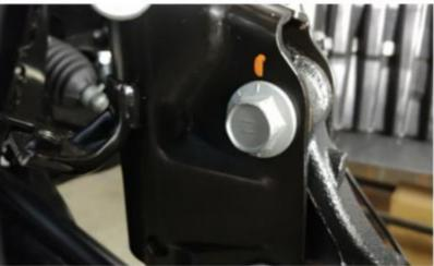
Re-attach brake line bracket in original location using factory hardware. Torque to 5 ft-lbs.
