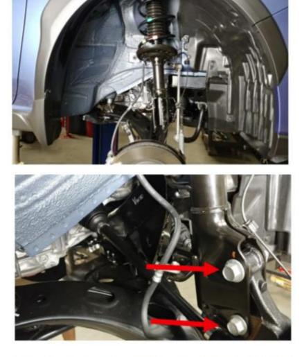
Raise the knuckle up and install into the strut body. Install the cam bolt into the upper hole and the remaining bolt into the lower.
