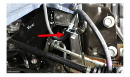
Remove the ABS harness clip at the strut body. Let hang out of the way.
