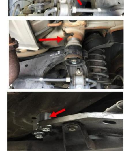
Raise the lower control arm into place and install the lower strut hardware. Do not tighten at this time. Use the jack and raise the lower control up to set preload on the strut. Install the lower knuckle bolt. Torque to 95 ft-lbs.
