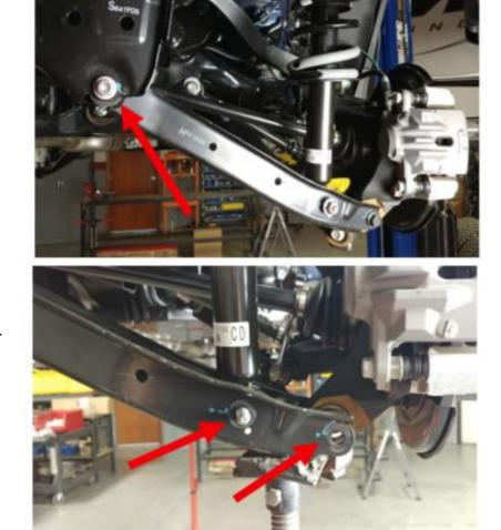
Support the strut and lower control arm, remove the lower strut and knuckle bolts. Lower the control arm down, while holding the strut. Remove the strut from the vehicle. A helper is recommended to hold the strut from falling.
