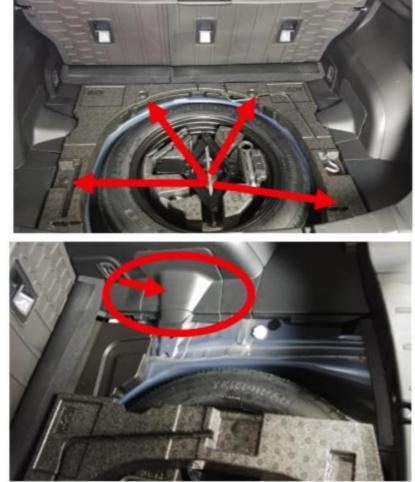
Remove these clips and set the foam pieces aside. Remove the strut covers by pulling upwards at the trunk area, then pushing down at the plastic cover, and set aside.
