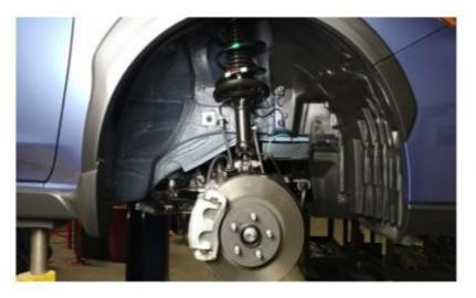
Remove the brake line bracket at the strut body. Let hang out of the way. Note how the brake line is run from the underside of the strut body. Installation will be changed in a later step.
