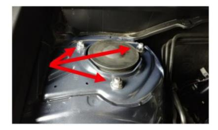
Locate the front strut extension. Passenger side shown. Install to the top of the strut using the factory hardware. Torque to 30 ft-lbs.
