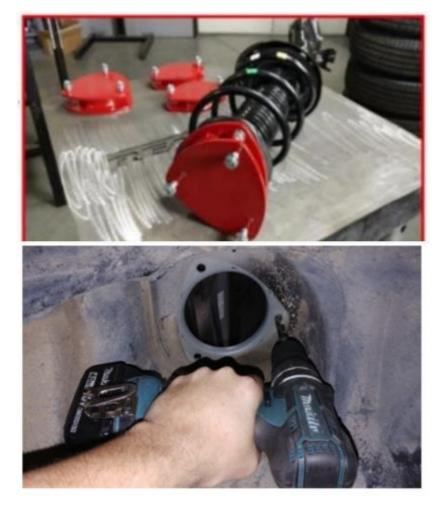
Drill out the 6 strut mounting holes in the strut tower with a 27/64" drill bit. Paint exposed metal with a high quality rust preventative paint. (Shown drilling from the wheel well due to the cowl overlap. DO NOT drill into the cowl or any harnesses. A drill stop is recommended.)
