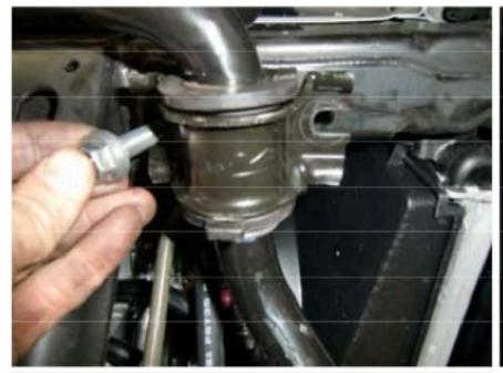
Remove the sway bar from the frame on both sides. Remove the metal saddle and leave the bushing.
