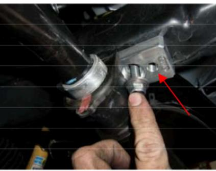
Install aluminum spacer to the frame using the hardware supplied. Note the position of the holes.
