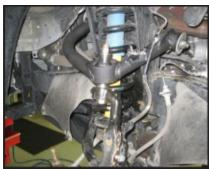
10. Working on the driver side, locate 1/4" nylock nut and 1/4" USS flat washer. Attach the OE ABS brake wire bracket to the new upper control arm. Repeat on passenger side.
