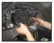
6. Locate the new upper control arms. Install the new bushings and sleeves into the new upper control arms. Special note: Make sure to use a fair amount of lithium or moly base grease before installing the new bushings and sleeves into the control arms. This will increase the life of the bushing as well as help prevent squeaking.
