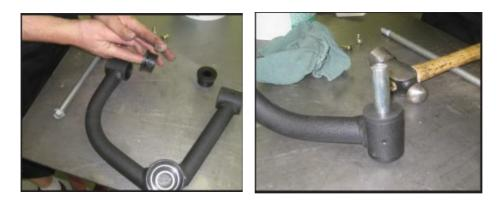
7. Locate the new sert fittings. Install the new sert fittings into the new upper control arms. Special note: Make sure not to over tighten and also make sure that the sert fitting is facing towards the outside of the vehicle. This will make for easier access when using a grease gun.
