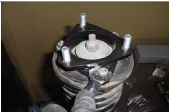
Attach new strut extension with OE hardware
