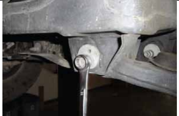
Reset and tighten lower control arm bolts
