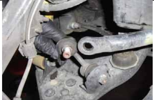
Disconnect both sides sway bar end links
