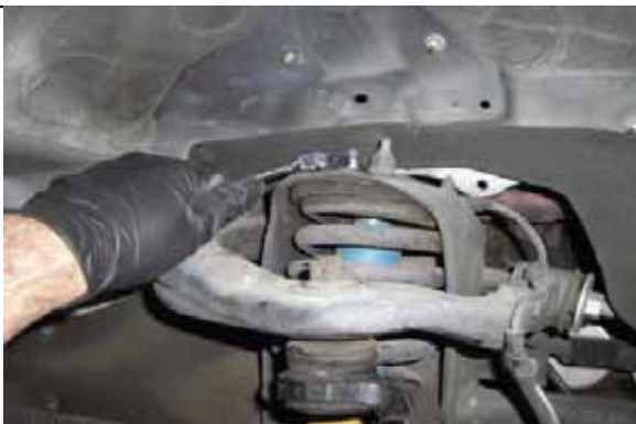
Disconnect upper strut mounting hardware
