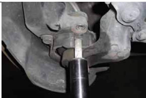
Disconnect lower ball joint hardware bolts
