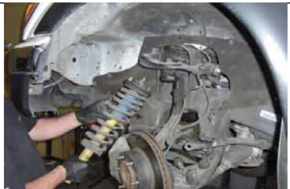
Remove strut from vehicle
