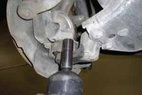
Reattach lower ball joint bolts and tighten
