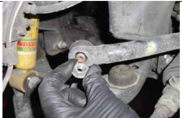
Reconnect sway bar end links. Move to the rear installation
