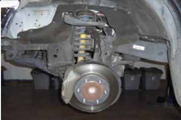
Raise and support vehicle by frame
