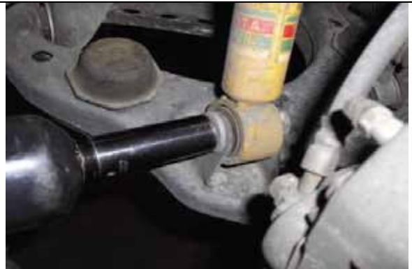
Disconnect lower strut mounting hardware
