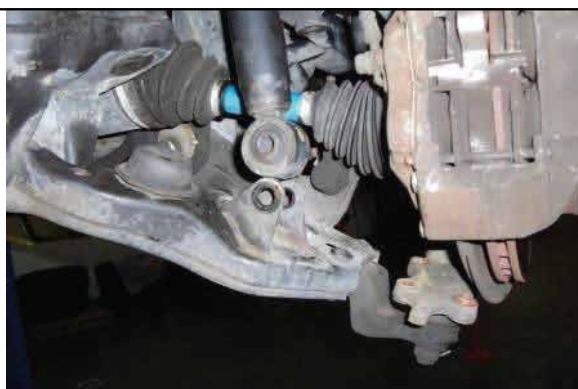
Lower control arm if necessary to install lower mount
