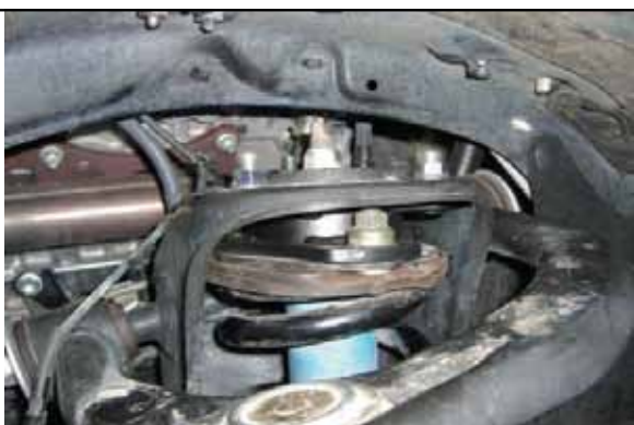
Rotate 180 deg., reattach upper strut with provided hardware
