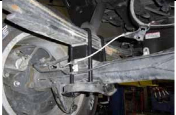
Attach lower mounting plate with provided hardware.
