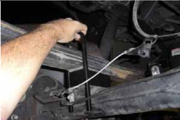
Slide new u-bolts over leaf pack and bumpstop bracket.
