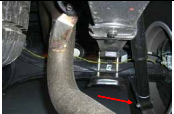
Remove rear lower shock bolt and disconnect shock.
