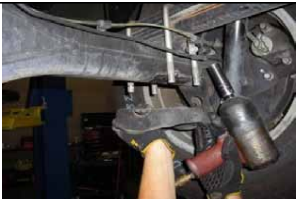
Remove u-bolt nuts and lower plate.
