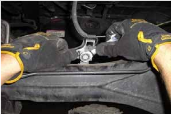
Replace shock on mount and ABS line to axle.
