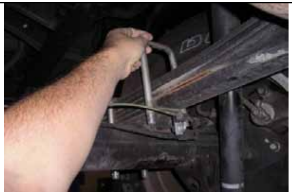
Carefully lower axle and remove u-bolts
