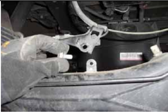
Disconnect ABS wiring brackets from axle.
