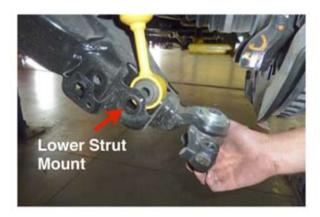
Lower strut being properly aligned with the lower strut mount.
