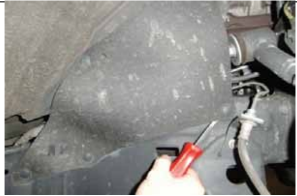
Remove splash guards at frame behind upper control arms.
