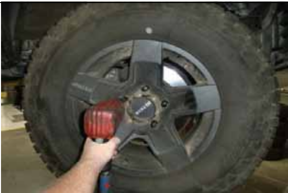
Reinstall wheels/tires and lower to ground.
