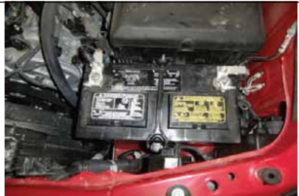
Disconnect positive/negative terminals and hold down clamp.
