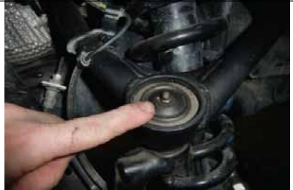
Make sure to grease ball joints and control arms.
