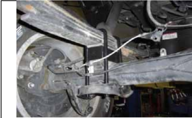
Attach lower mounting plate with provided hardware.
