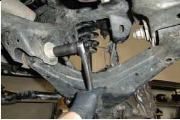
If lower control arm bolts were loosened, retighten now.
