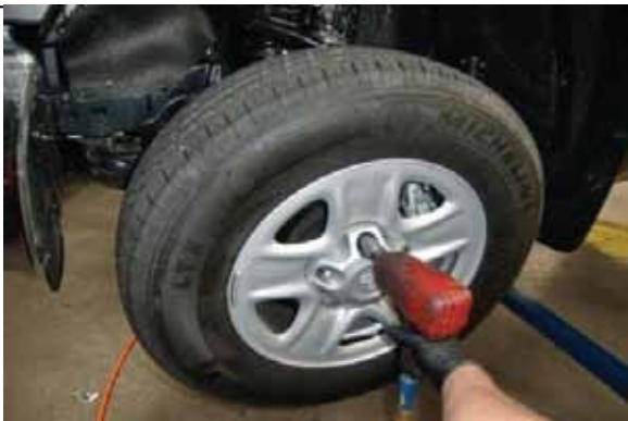
Remove wheels/tires from vehicle.
