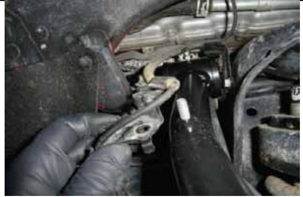
Attach ABS line to upper control arm with provided hardware.
