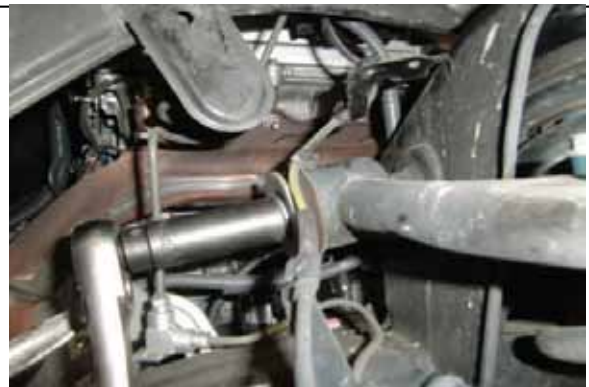
Loosen upper control arm and remove, use caution.
