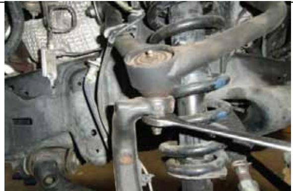
Raise suspension and reattach upper ball joint to spindle.
