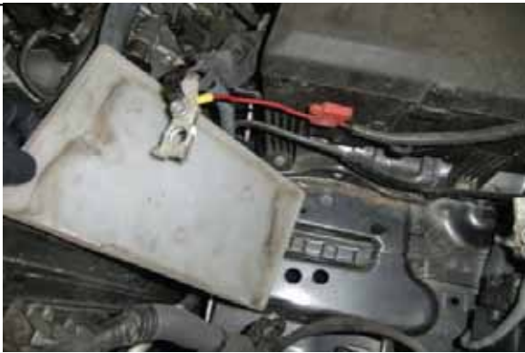
Remove battery and plastic tray from truck .
