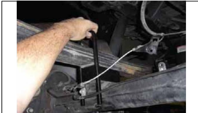
Slide new u-bolts over leaf pack and bump stop bracket.
