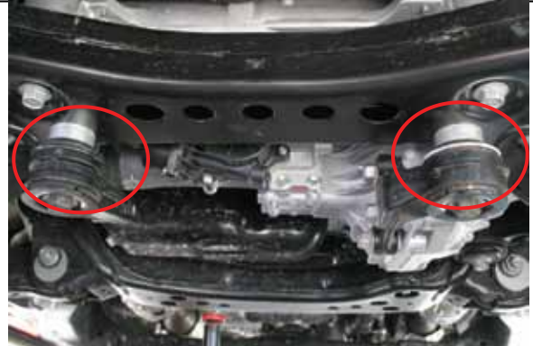
4WD Install new longer bolts to reattach and tighten.
