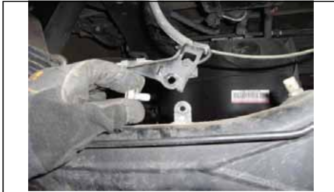
Disconnect ABS wiring brackets from axle.
