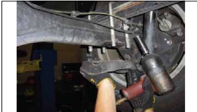
Remove u-bolt nuts and lower plate.
