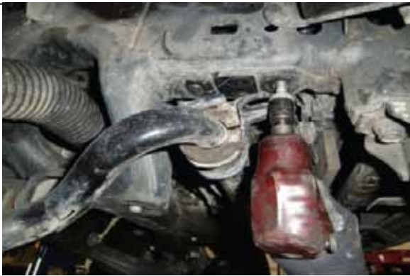
Disconnect sway bar at the frame mounts.
