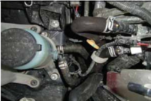
Disconnect wiring loom and hose clamp on passenger side.
