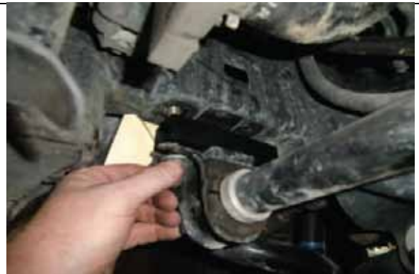
Now install sway bar drop brackets at frame w/new hardware
