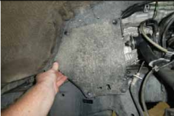
Reinstall the splash guards (4) removed in the initial steps.
