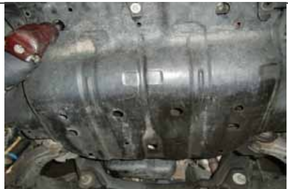
Remove front skid plate to expose sway bar.
