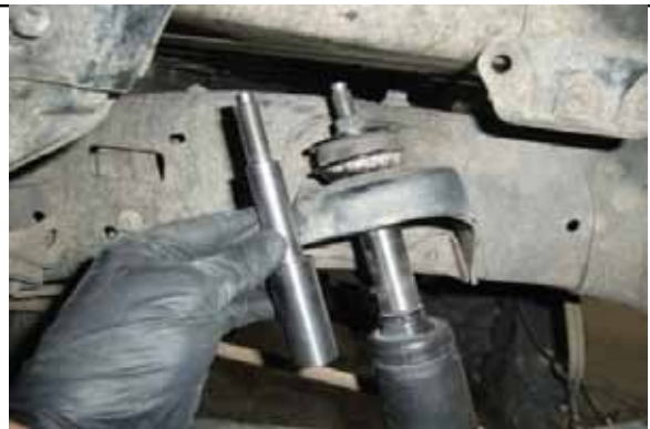
Install provided upper shock extension as shown.
