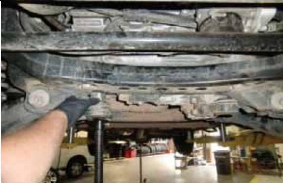
4WD Slowly lower to allow spacers to be placed as shown.
