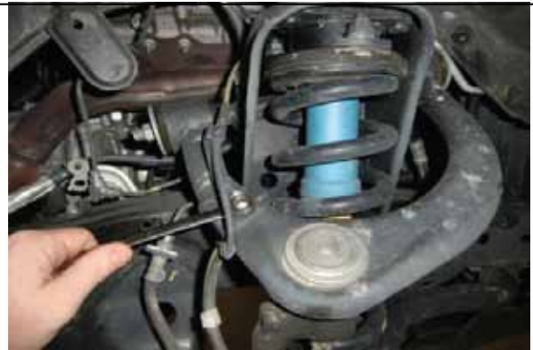
Unbolt ABS line bracket on top of upper control arms.
