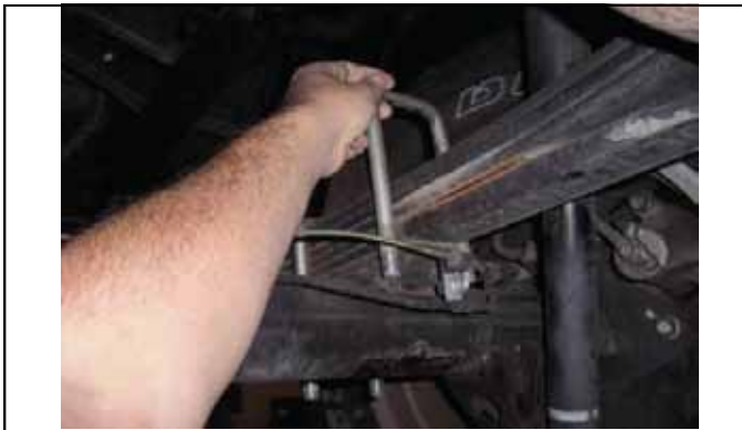
Carefully lower axle and remove u-bolts
