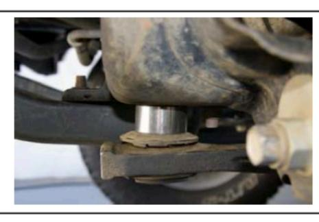
3. Install the 1" spacers between the differential supports and the front cross-member. Install the new bolts with factory washers and the new nuts and washers.
