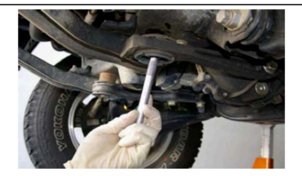
2. Remove the factory 19mm differential mounting nuts and bolts. The OEM washers will be reused.
