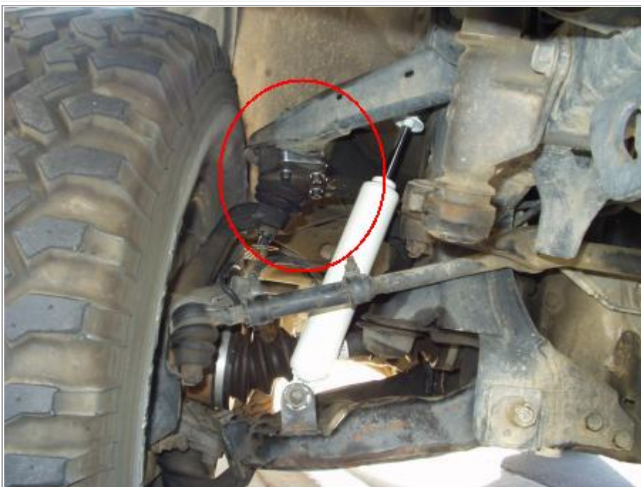
Ball Joint Spacer Installation
