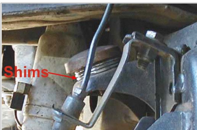
Shimming for low profile bump stops
