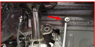
Support the lower control arm with a suitable jack.
