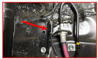
Install the sway bar bracket to the strut using the provided
