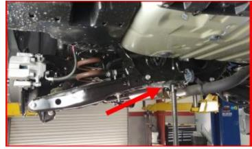
Locate the cradle stud inside the rear spring.
