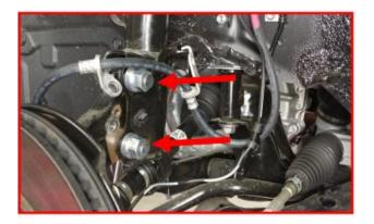
Install the tie rod end to the knuckle using the factory hardware.
