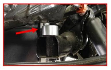
Install the ABS drop bracket to the frame using the factory hardware. Install the ABS factory bracket to the drop bracket using the provided 1/4" bolts, washers, and nuts. Torque to 5 ft-lbs.
