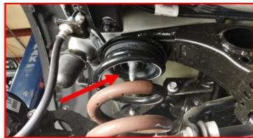
Unscrew the nut until it reaches the end of the stud.
