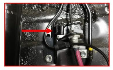
Remove the ABS wire and brake line bracket from the strut body. The ABS bracket sits in front of the brake line bracket. Open the plastic clip on the strut to remove the ABS wire from this point. Let all hang out of the way. Remove the brake line bracket at the knuckle.
