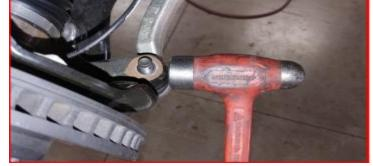
Remove the sway bar end link from the strut. Let hang out of the way.
