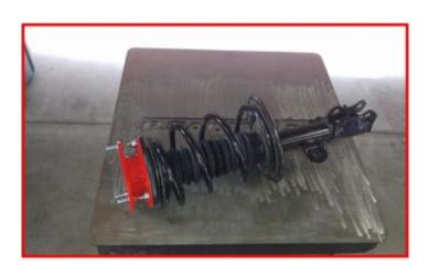
Install the completed strut assemblies into the strut tower using the factory hardware. Do not tighten at this time.
