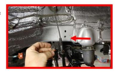
Under the driver side locate the fuel filler shield.
