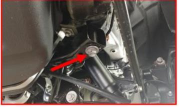
Locate the cradle spacers. The round will go in the front location and the square slotted spacers will go in the rear location above the springs.
