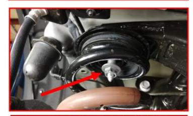
Locate the front cradle bolts. Remove these completely and discard hardware.
