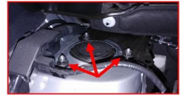
Remove the strut from the vehicle. Be careful to not dislocate the cv shafts from their housings. If this happens, carefully push the CV axle back into the cup. You may have to rotate the hub at the same time.
